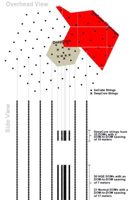
Figure 3. Schematic view of the IceCube Neutrino Observatory including the low energy extension DeepCore. Shown in red is the partially instrumented detector, which was the only portion used in the reviewed paper. Reprinted from [1].
